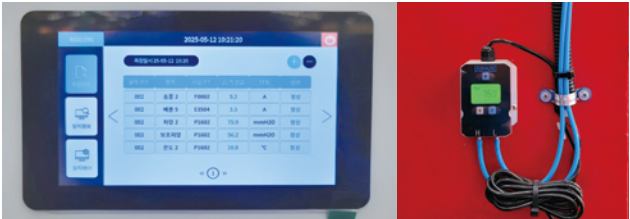
IoT Device for Air Quality Monitoring on Coating Equipment (Dong-A Steel)
