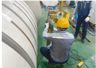
Non-Destructive Testing (NDT) of Crane Attachment Equipment (SeAH Steel Changwon Plant)
